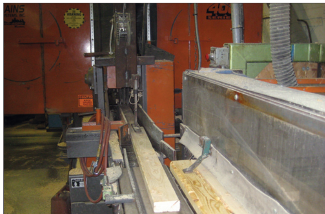
Infeed of West Plains 400 series band resaw, which is set up to split 2x4 material.
