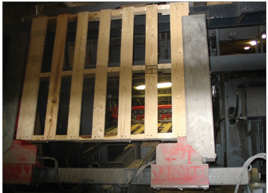
After one deck is nailed, the Storti Flex 2600 automatically advances the pallet and turns it over in preparation for the final components to be placed into position and nailing the second face.
