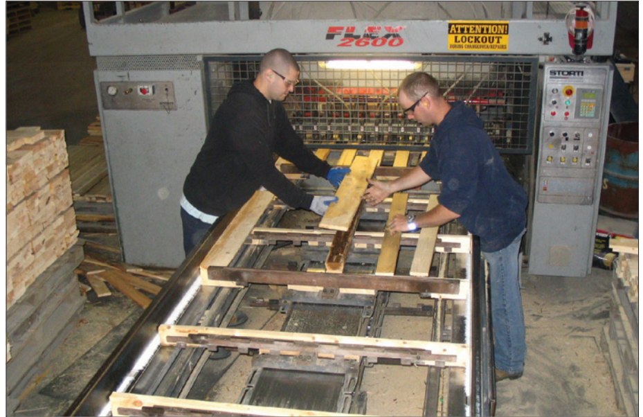
Workers at Bluewater Pallet place pallet parts into Storti Flex 2600 nailing machine; the Flex 2600, which assembles stringer pallets with ‘beam’ nailing orientation, also can nail block pallets.
